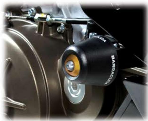
SEARCH AND FIND THE FIXING POINT ON THE MOTORBIKE, USE THE SPECIFIC THICKNESS AND BOLTS LIKE DESCRIBED IN THE PICTURE (SO YOU CAN GET THE RIGHT PROMINENCE FROM THE MOTORBIKE). FIX THE PVC HEAD AFTER FIXED AND TIGHTEN ALL THE KIT ONLY.
