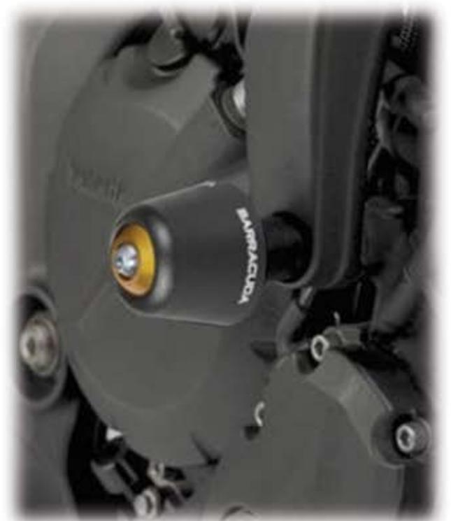
SEARCH AND FIND THE FIXING POINT ON THE MOTORBIKE BEFORE START TO MOUNTAIN, USE THE SPECIFIC THICKNESS AND BOLTS LIKE DESCRIBED IN THE PICTURE (SO YOU CAN GET THE RIGHT PROMINENCE FROM THE MOTORBIKE).
